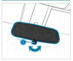
To dim the inside rearview mirror: move anti-glare lever in in the direction of the arrow.
