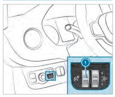
Turn brightness control knob () upwards or downwards.
