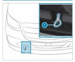
Installing and removing the front towing eye
