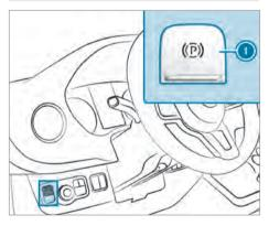
**To apply:** press switch **()**. When the electric parking brake is applied, the red **PARK** and **(@)** (USA) or **(@)** (Canada) indicator lamps light up in the instrument display. The electric parking brake is only actually applied when the red **PARK** and **(@)** (USA) or **(@)** (Canada) indicator lamps light up continuously.
