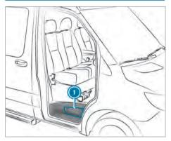
The hydraulic jack is located in side compartment above the co-driver door step.
