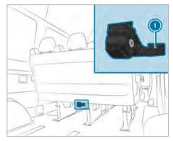
Tilt the bench seat forwards firmly until the locks on the front legs of the bench seat engage audibly.
