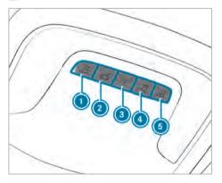
Switches the front left reading lamp on/off
