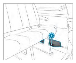
Depending on the vehicle equipment, there will be an air duct or a heater with additional air vents in the rear compartment footwell on the left-hand side (). No objects may be placed there. Occupants must maintain a sufficient distance due to the warm air flow and air intake.
