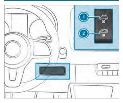
If your vehicle is equipped with a roof ventilator, you can admit fresh air to the cargo compartment, or extract air from it as well.
