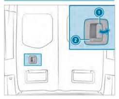
The  $\square$  symbol indicates that the rear-end door is unlocked.
