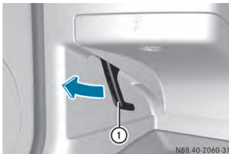
Hood release lever in the driver's footwell
