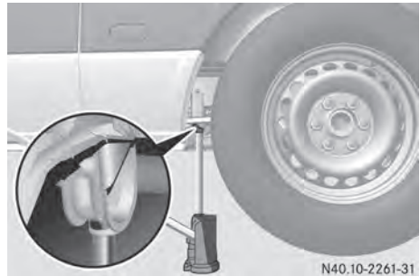
Jacking point, rear axle (example: vehicle type 2500)
