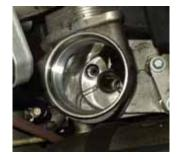
There have been several discussions as to whether there is a mess in pulling the filter from the block-integral oil filter canister. That is not the case. The oil drains directly into the block. Note the condition of the canister upon removal of the filter.
