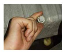
Drain the oil. There have been discussions whether through-the-dipstick oil removal, as used on other Mercedes engines, works. I jerry rigged a system to test it out – I was not successful. It left 1.5 qts behind.
