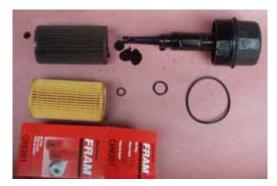
Pull the old filter off and remove the three Orings from the plastic filter mounting spike. Replace with new Orings provided in the new filter kit. Then slide the new filter onto the mounting spike.
